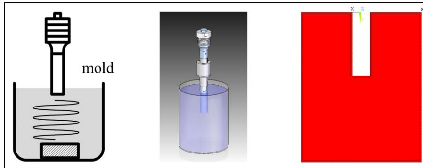
Figure 3: Left: Sketch of experimental setup; Centre: Experimental setup as CAD drawing; Right: Two-dimensional geometry modelling the fluid for finite element computations.
