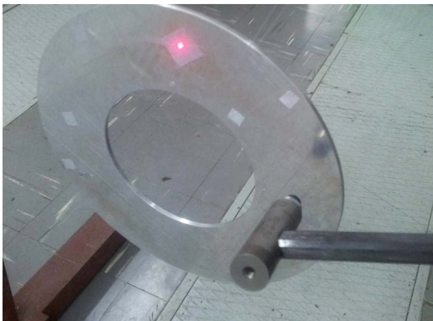
Figure 3: Modal testing using hammer blow for excitation and laser velocimeter for measurement (red point).
