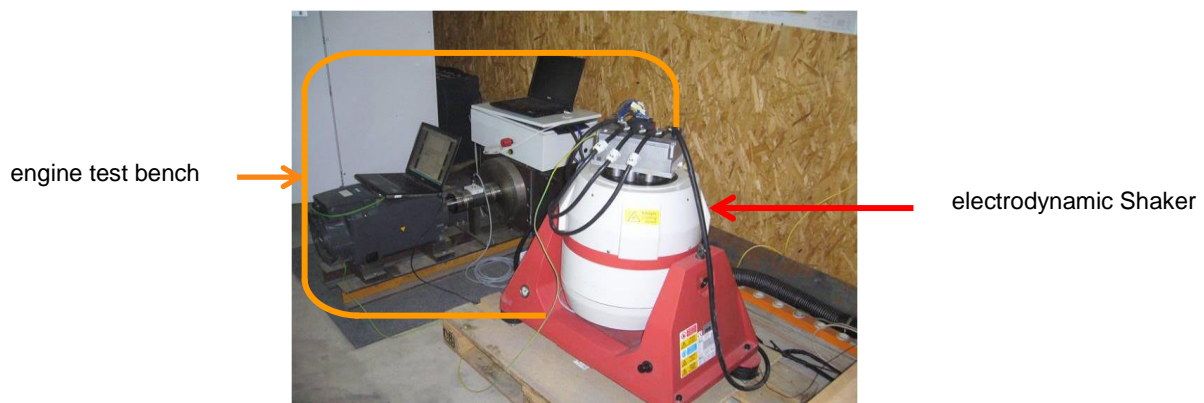
Figure 5: Drive control stressed by vibrations and shocks with applied supply voltage of the traction battery.
