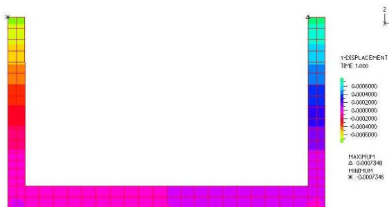
Figure 6: Horizontal displacement given from hand made hydrostatic pressures
