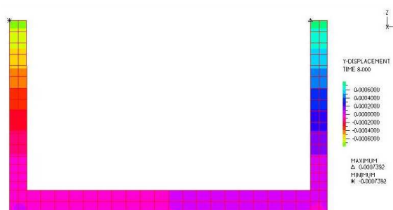
Figure 7: Horizontal displacement by using FEM ALE FSI in time t = 8 s (only hydrostatic effect)
