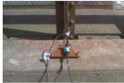
Figure 6: Schematic representation of the measurement points in the cross sections of spans 1, 2 and 3 and the position of the accelerometers in one of the instrumented point.
