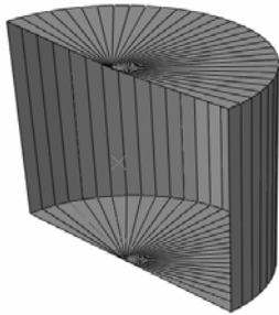
Figure 3. 180 ° axisymmetric model of auxiliary chamber
