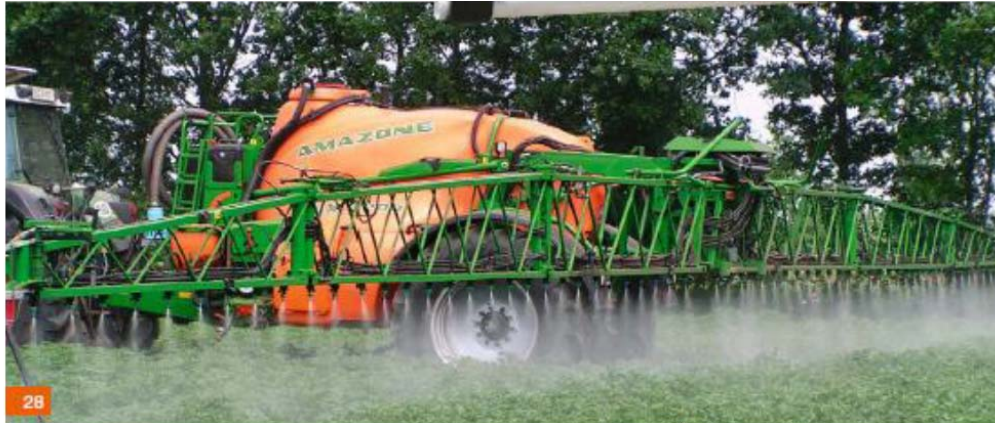
Figure 1: Spray boom UX-5200 from Amazone [9].
