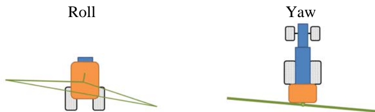
Figure 3: Spray Boom Movement.
