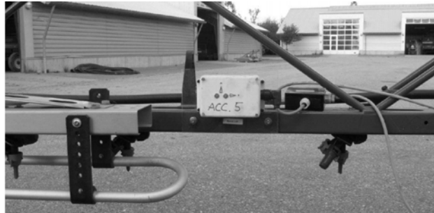
Figure 6: The accelerometer mounted on the spray boom.
