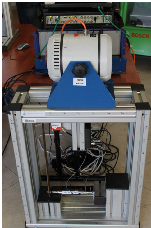
Figure 10: Model equipped with electrodynamic exciter
