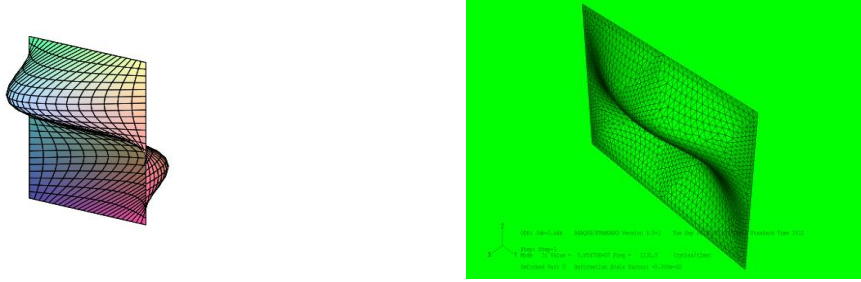
Figure 4. Comparison of Mode 3 shape for (\alpha, \beta) = \left(\frac{1}{2}, \frac{1}{2}\right) . Left: Galerkin, Right: ABAQUS.
