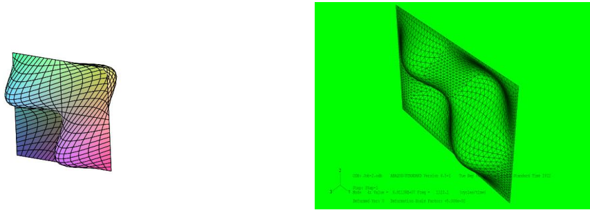
Figure 5. Comparison of Mode 4 shape for (\alpha, \beta) = \left(\frac{1}{2}, \frac{1}{2}\right) . Left: Galerkin, Right: ABAQUS.
