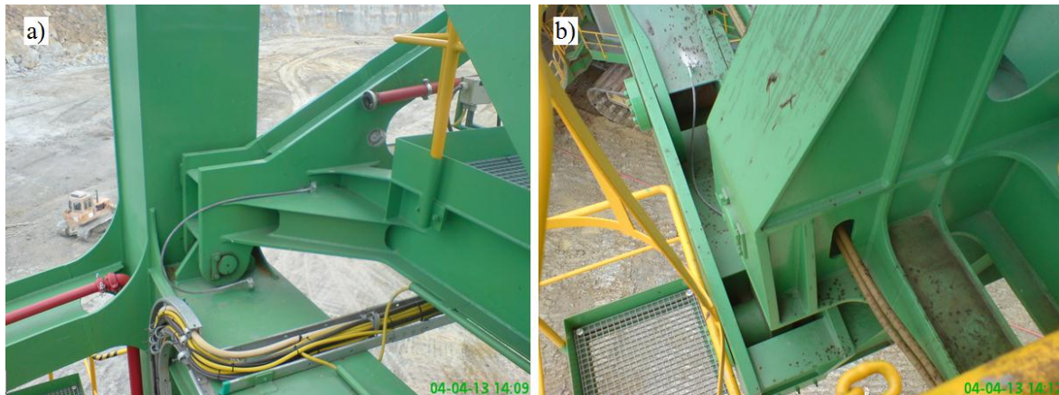
Figure 5: The final design of the counterweight boom supporting system: front a); rear support b).
