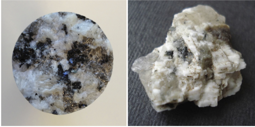
Figure 6: Riverina granite (left) vs. Habanero granite sample (right). High percent of quartz content is observed in both samples.
