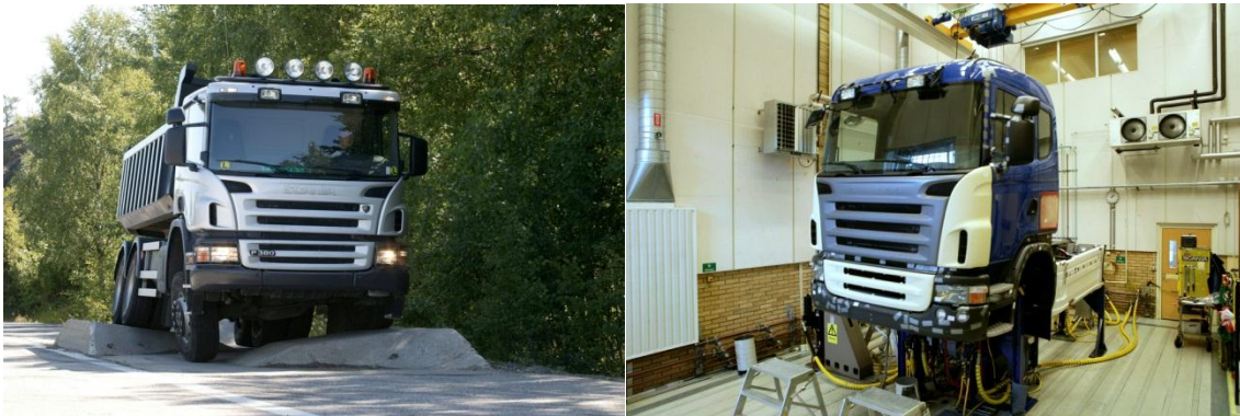
Figure 1: a) Photograph of a vehicle on the test track in Södertälje. b) Photograph of a test rig at Scania AB that aims to reproduce the damage of the test track.
