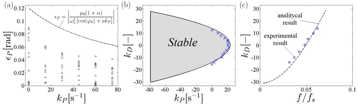
Figure 6: (a): Error in the positioning of the pendulum.  $\triangle$  experimental results; dashed line: analytical result ( $\mu_0(1 + \alpha) = 4.6 \text{ rad/s}^2$ ). (b): stability chart for  $\tau = 0.05 \text{ s}$ ,  $r = 1$  and  $\varphi_0 = 0.64 \text{ rad}$  (as in Fig. 4(b)). (c): frequency of oscillation at the loss of stability; dashed line: analytical result, blue squares: experimental results.
