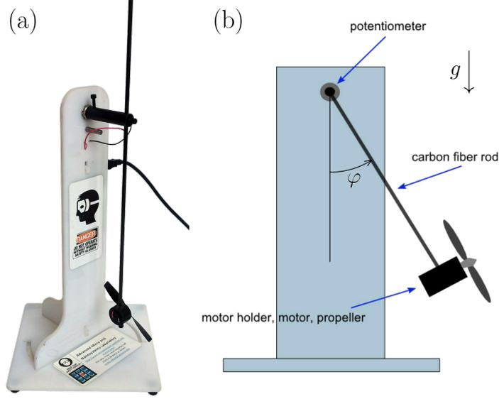
Figure 1: (a): Aeropendulum (photo); (b): schematic physical model
