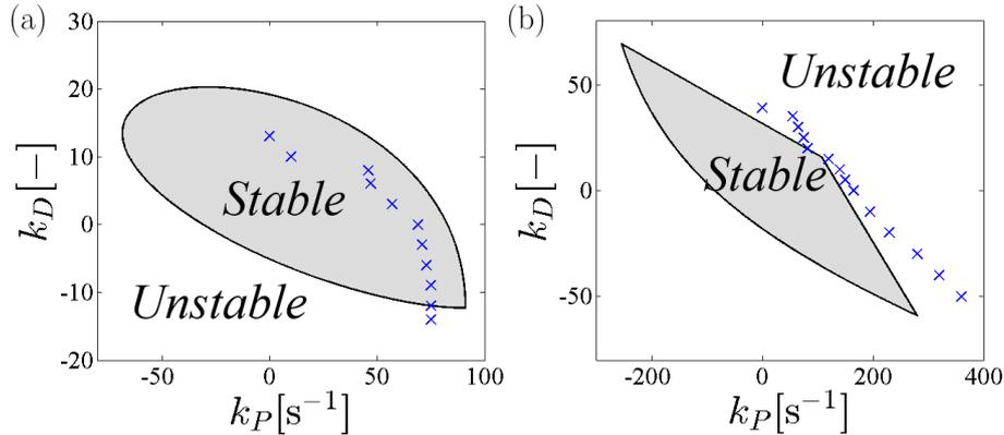
Figure 5: Stability chart of the system in Eq. (7) around the point  $\varphi_0 = 0.64$  rad. (a): normal controller; (b): act-and-wait controller.  $\tau = 0.3$  s,  $r = 2$ . Blue  $\times$ -s refer to the experimental right border of stability.
