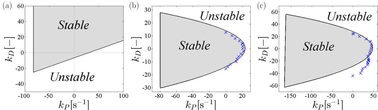
Figure 4: Stability chart of the system in Eq. (7) around the point  $\varphi_0 = 0.64$  rad. (a): continuous time approach (or  $\tau \rightarrow 0$ ); (b): discrete time,  $\tau = 0.05$ ,  $r = 1$ ; (c): act-and-wait controller,  $\tau = 0.05$ ,  $r = 1$ . Blue  $\times$ -s refer to the experimental border of stability.
