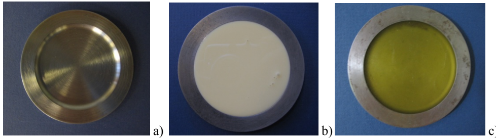
Figure 1: Samples for impact tests: a) DH-36 steel plate's geometry; b) steel plate coated with alumina particle-polyurea ( V_f=5.7\% ) composite and c) steel plate coated with milled glass-polyurea ( V_f=9\% ) composite.
